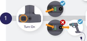
If battery level is low, the Ring Cutter can be operated plugged-in.
